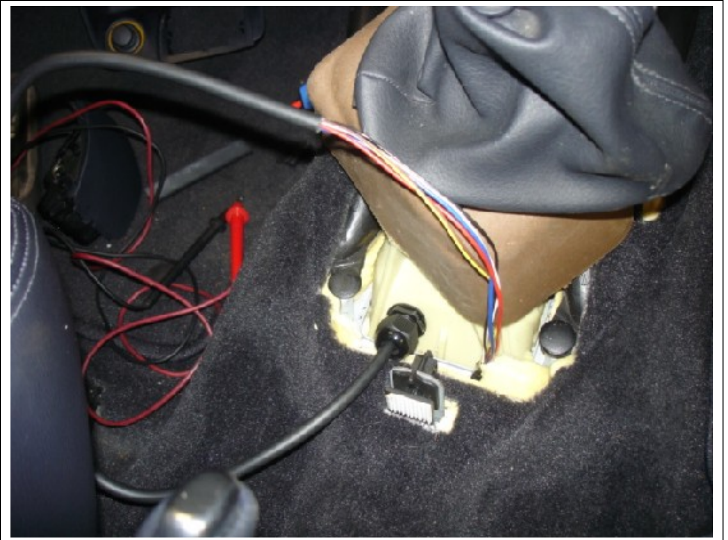
Feeding in the cable loom through the cable gland
